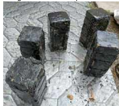
Figure 4 Bitumen coated flyash bricks.
