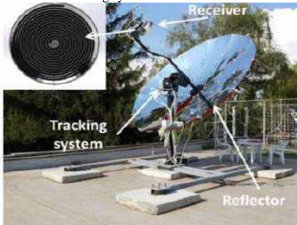
Figure 2 Parabolic dish collector system
