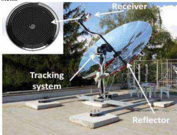
Figure 2 Parabolic dish collector system
